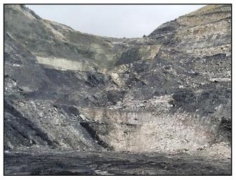
twenty named seams and the basin showed all the seams in the sequence. The present seam being worked is the Lochgelly Splint. There is a major fault running east to west through the site and the geology is further complicated by a syncline with the axis dipping to the south steepening up as you go down the sequence. In addition there is a dolerite sill which was full of serpentinite veins which made it difficult to work but it was being quarried for use as aggregate.
