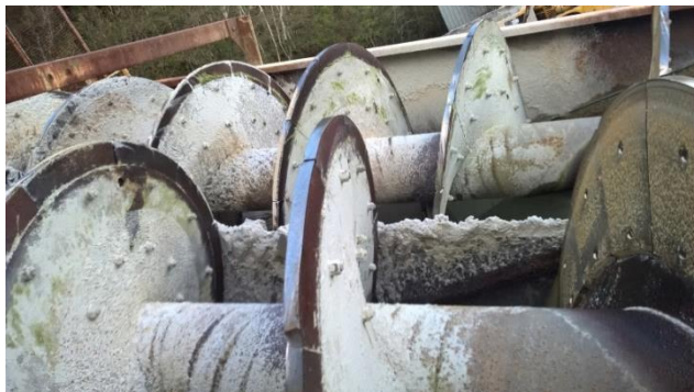
An Archimedes Screw used to lift the sand and water slurry.
